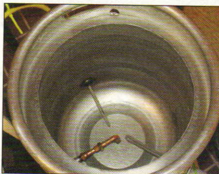
This kettle is dually heated with separate heating elements, giving it the capability to bring wort to a boil, then shut one down.
