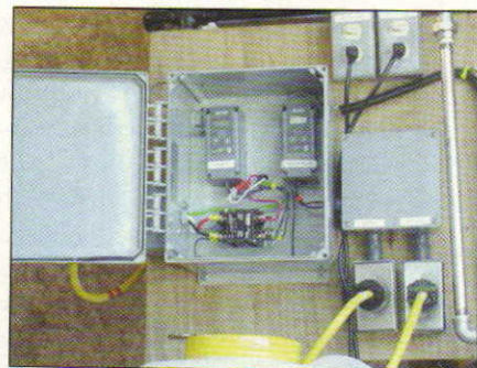
Steve added two electric temperature control elements for accurate and precise heating of his liquor tank and kettle.
