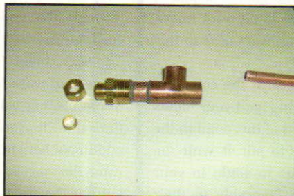
The copper tee, 1/2” copper pipe and compression fittings are assembled as shown. Use JB Weld to hold them together.
