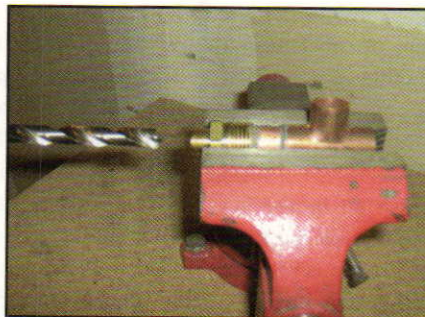
Use a drill with a 3/8” bit to ream out the tee fitting for the chiller. Place the fitting in a clamp to hold it securely.
